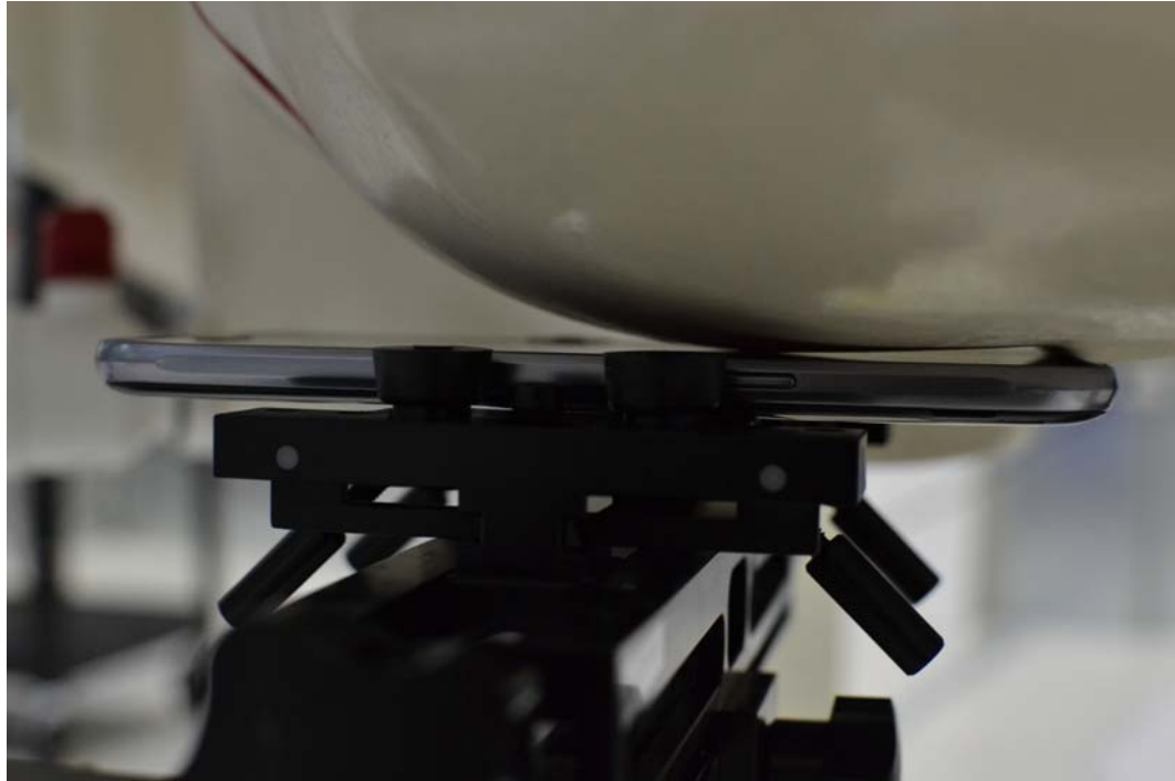
SAR Test Setup Photo 3 – Left Cheek
