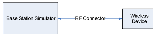
Figure 9-1 Power Measurement Setup
