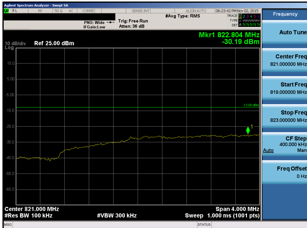
Plot 7-119. Lower Extended Band Edge Plot (Band 5/26 – 5.0MHz QPSK – RB Size 25)
