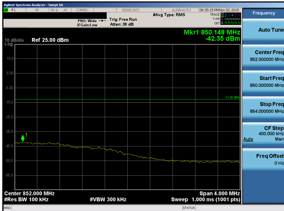
Plot 7-113. Upper Extended Band Edge Plot (Band 5/26 – 1.4MHz QPSK – RB Size 6)
