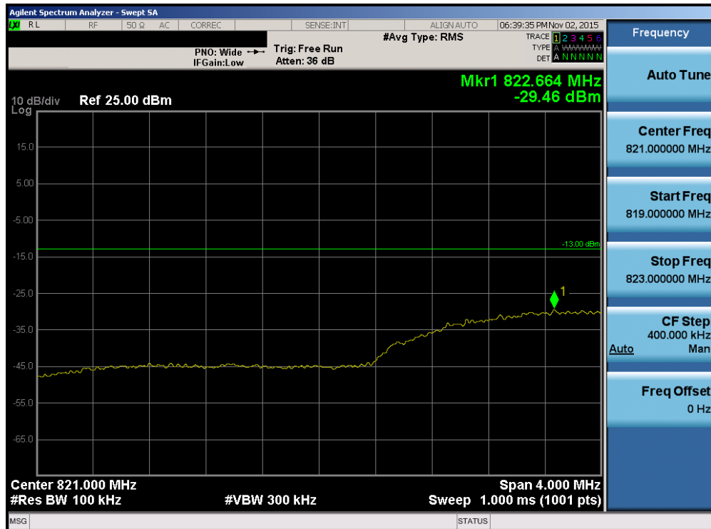
Plot 7-115. Lower Extended Band Edge Plot (Band 5/26 – 3.0MHz QPSK – RB Size 15)
