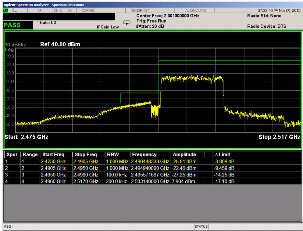
Plot 7-176. Lower ACP Plot (Band 41 – 10.0MHz QPSK – RB Size 50)
