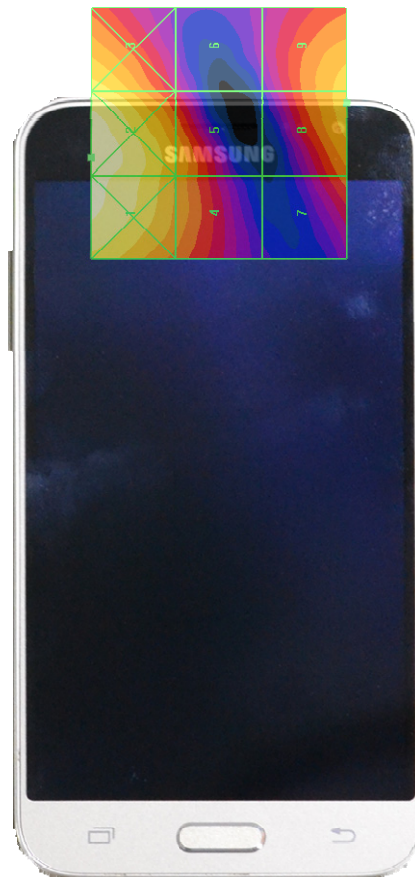
Figure 18-4 E-Field WD Scan overlay
