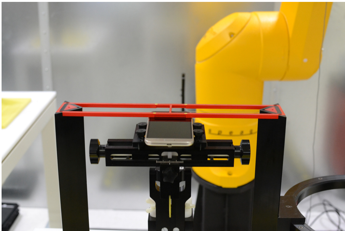
Figure 18-1 Ear Reference Point HAC Phantom Alignment
