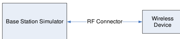
Figure 9-1 Power Measurement Setup
