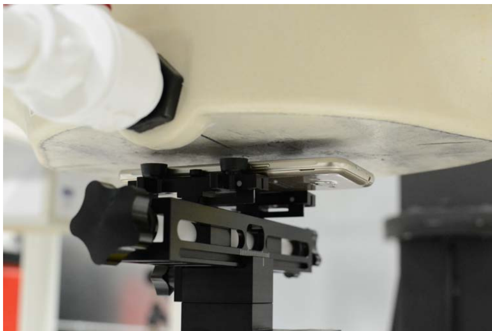
SAR Test Setup Photo 7 – Front Side at 10mm
