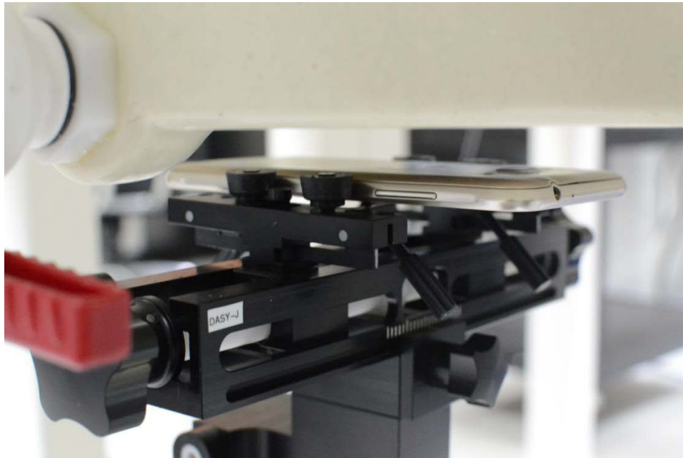
SAR Test Setup Photo 5 – Back Side at 15mm (Body-Worn)
