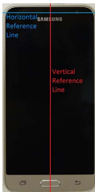
SAR Test Setup Photo 12 – DUT Reference Lines
