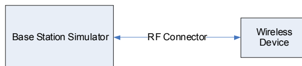
Figure 9-1 Power Measurement Setup
