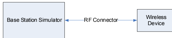
Figure 9-3 Power Measurement Setup
