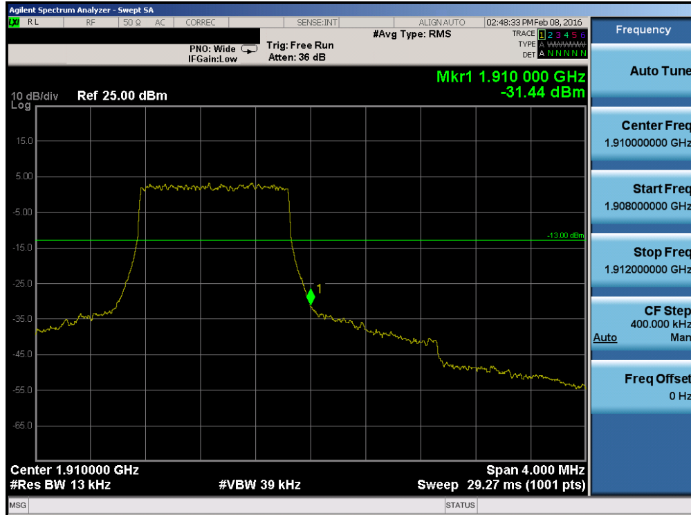
Plot 7-115. Upper Band Edge Plot (Band 2 – 1.4MHz QPSK – RB Size 6)
