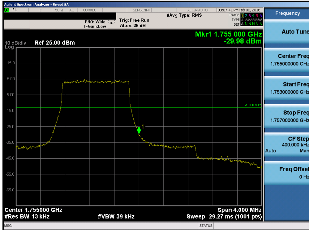
Plot 7-91. Upper Band Edge Plot (Band 4 – 1.4MHz QPSK – RB Size 6)
