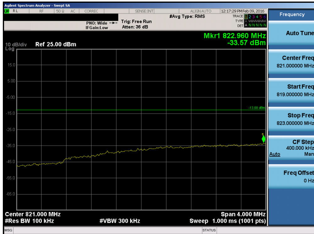
Plot 7-84. Lower Extended Band Edge Plot (Band 5 – 5.0MHz QPSK – RB Size 25)
