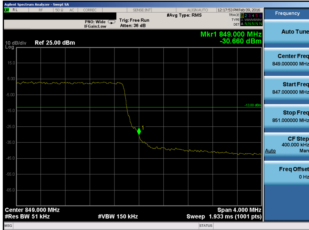
Plot 7-85. Upper Band Edge Plot (Band 5 - 5.0MHz QPSK - RB Size 25)
