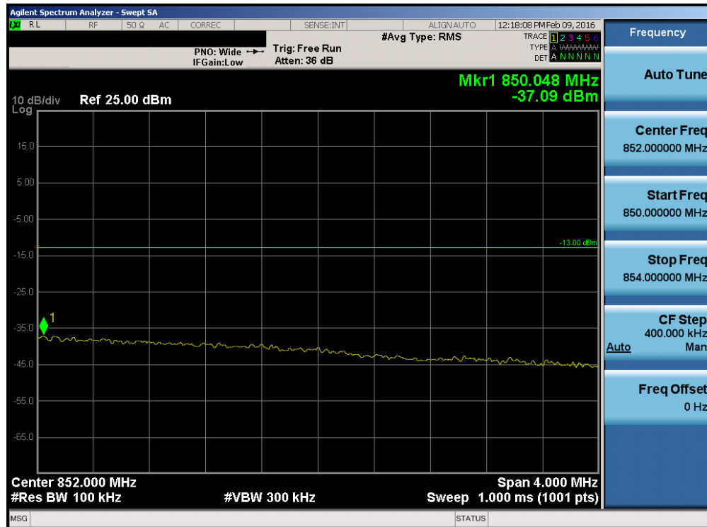
Plot 7-86. Upper Extended Band Edge Plot (Band 5 - 5.0MHz QPSK - RB Size 25)
