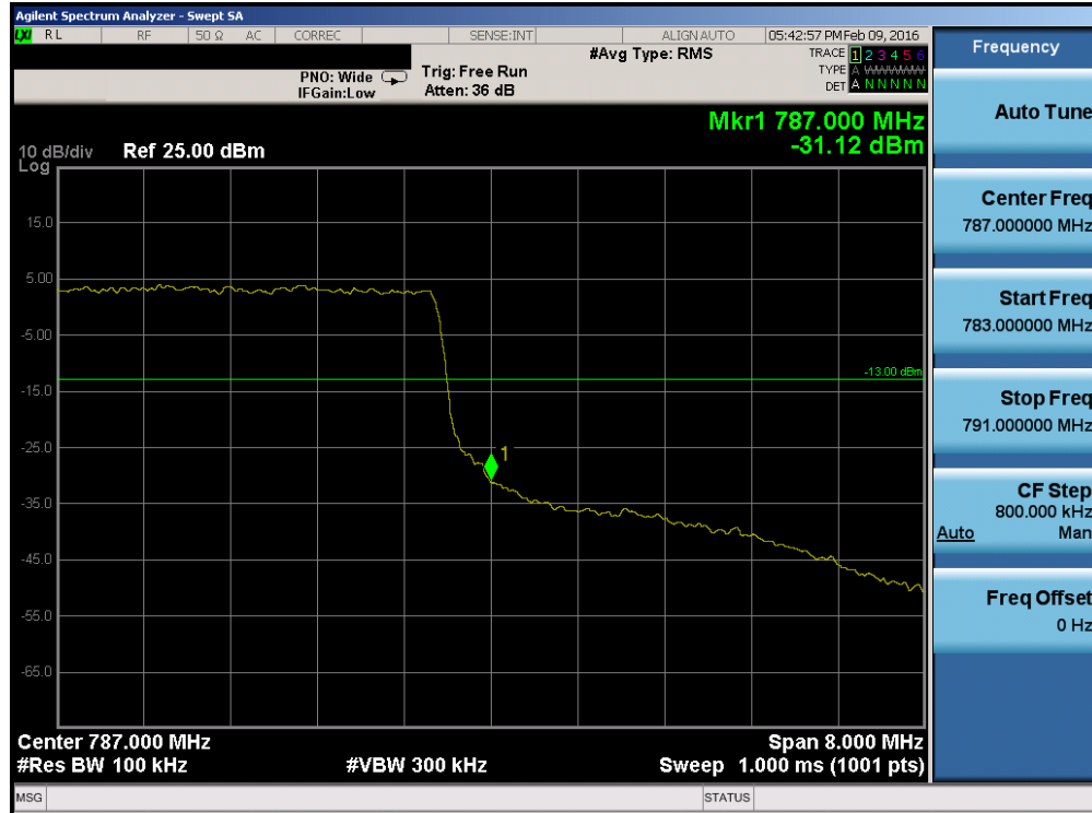
Plot 7-73. Upper Band Edge Plot (Band 13 – 10.0MHz QPSK – RB Size 50)
