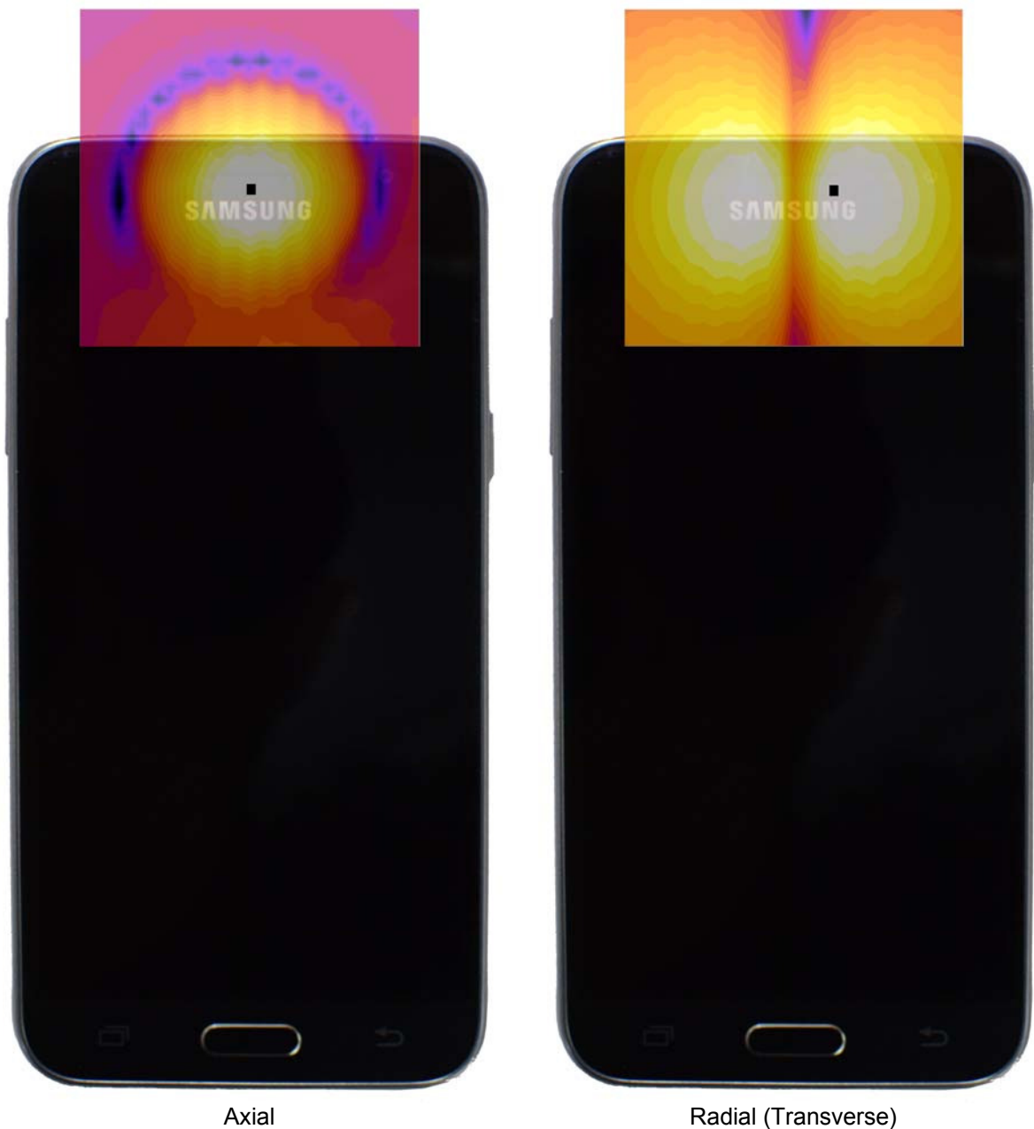
Figure 15-3 T-Coil Scan Overlay Magnetic Field Distributions
