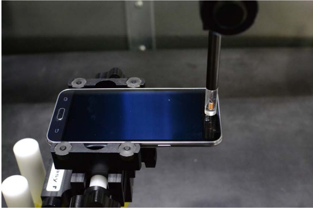
Figure 15-1 Test Setup for Wireless Device
