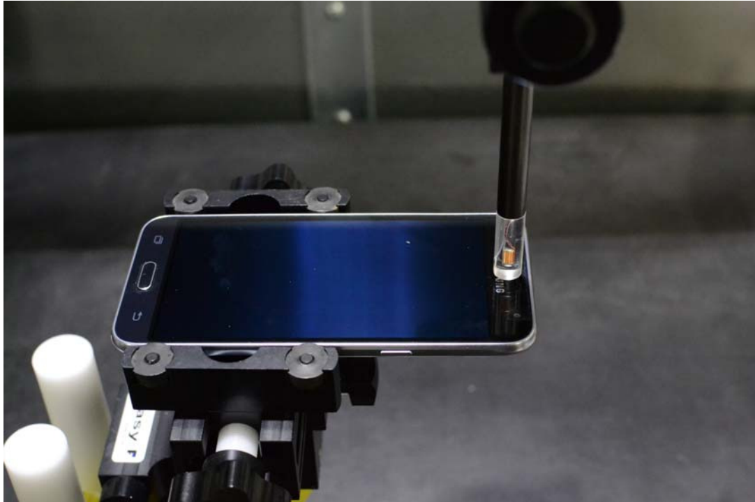
Figure 14-1 Test Setup for Wireless Device
