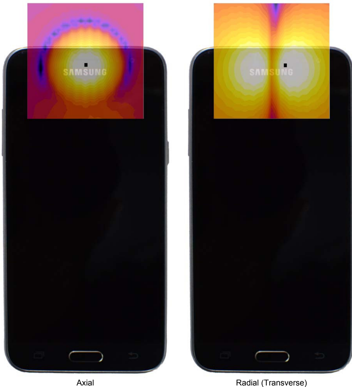
Figure 14-3 T-Coil Scan Overlay Magnetic Field Distributions
