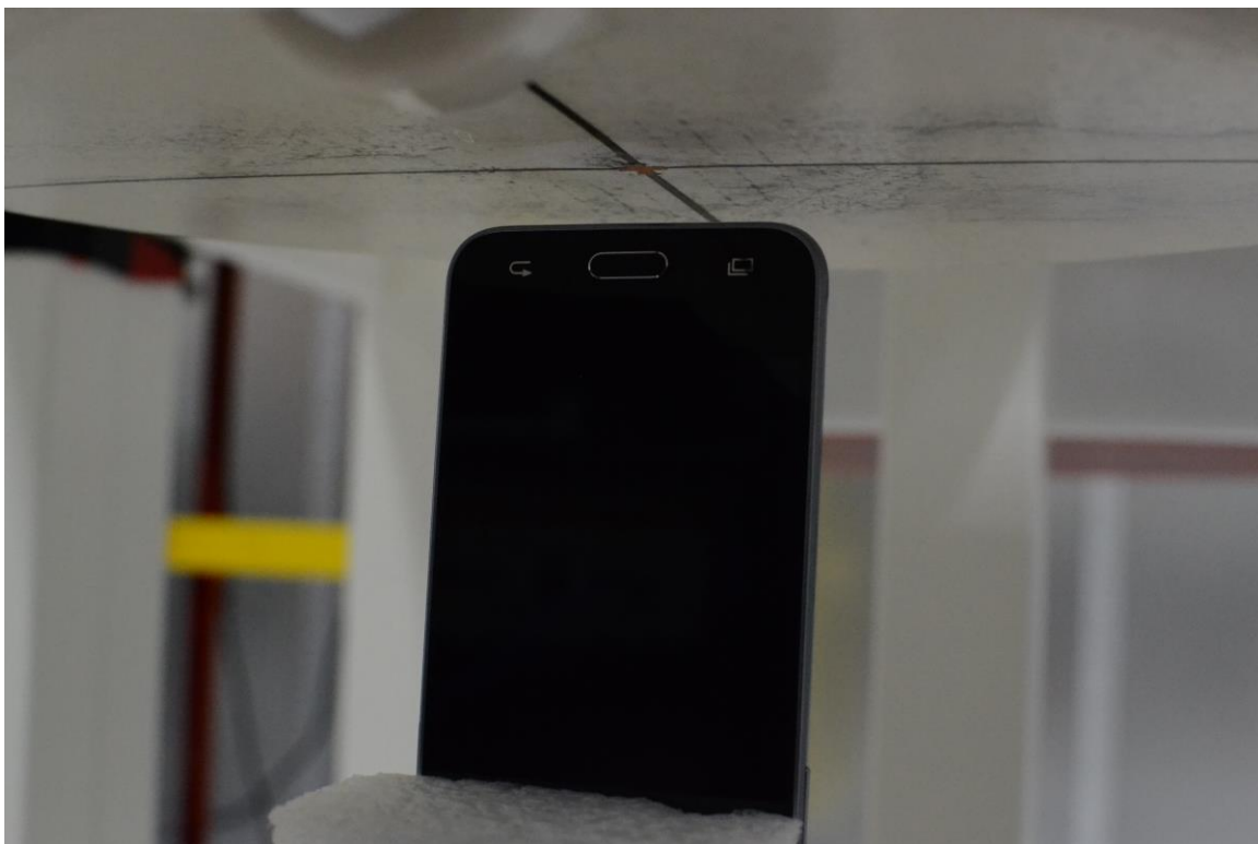
SAR Test Setup Photo 8: Bottom at 1.0 cm
