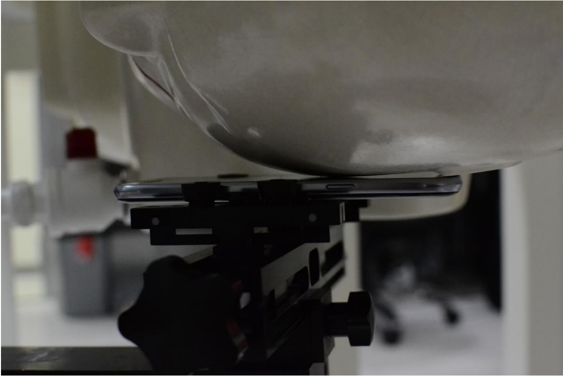
SAR Test Setup Photo 3: Left Cheek
