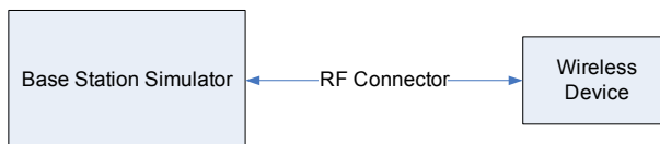
Figure 9-1 Power Measurement Setup
