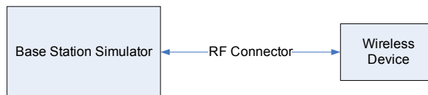
Figure 9-3 Power Measurement Setup
