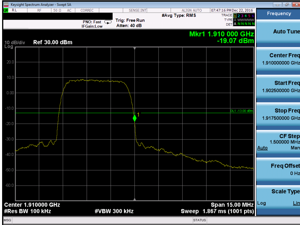
Plot 7-67. Band Edge Plot (PCS WCDMA Mode – Ch. 9538)
