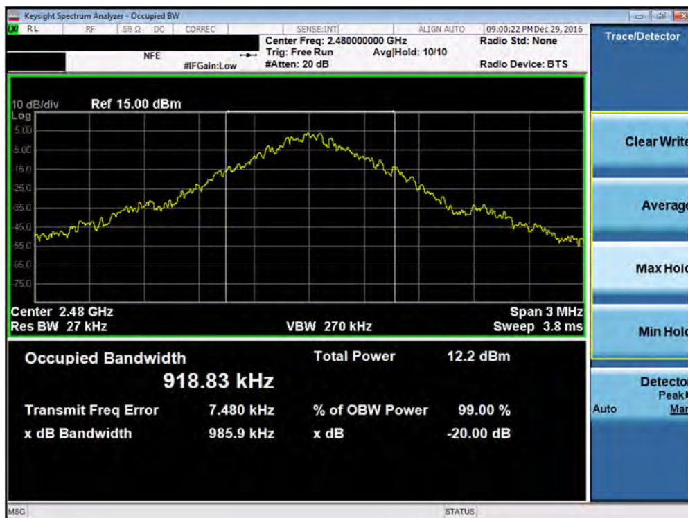
Plot 7-3. 20dB Bandwidth Plot (Bluetooth, 1Mbps – Ch. 78)
