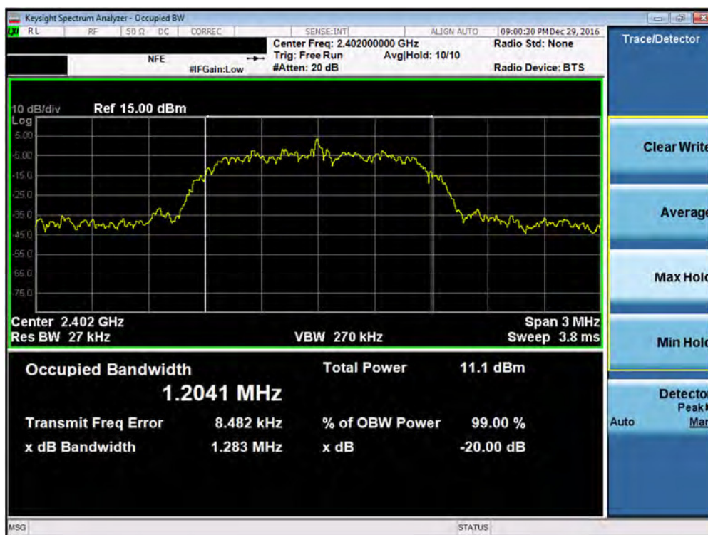
Plot 7-4. 20dB Bandwidth Plot (Bluetooth, 2Mbps – Ch. 0)
