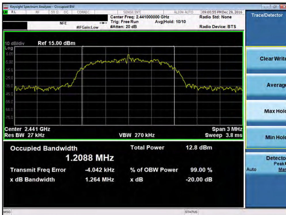
Plot 7-8. 20dB Bandwidth Plot (Bluetooth, 3Mbps – Ch. 39)
