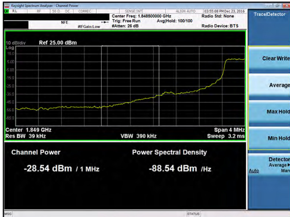
Plot 7-130. Lower Extended Band Edge Plot (Band 2 – 1.4MHz QPSK – RB Size 6)
