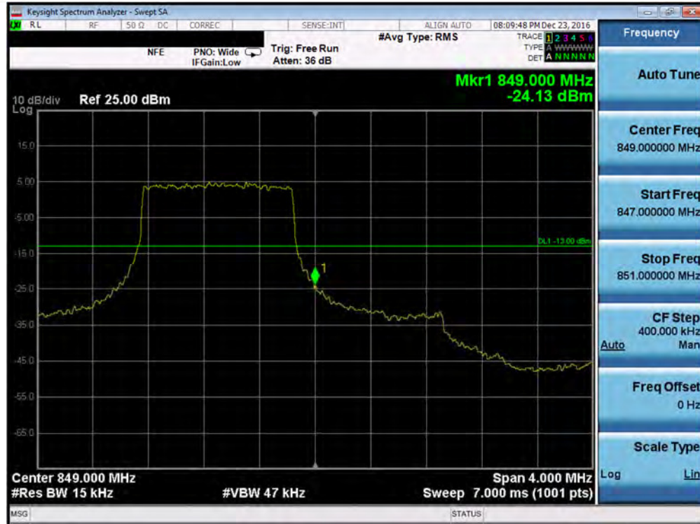
Plot 7-93. Upper Band Edge Plot (Band 5 – 1.4MHz QPSK – RB Size 6)
