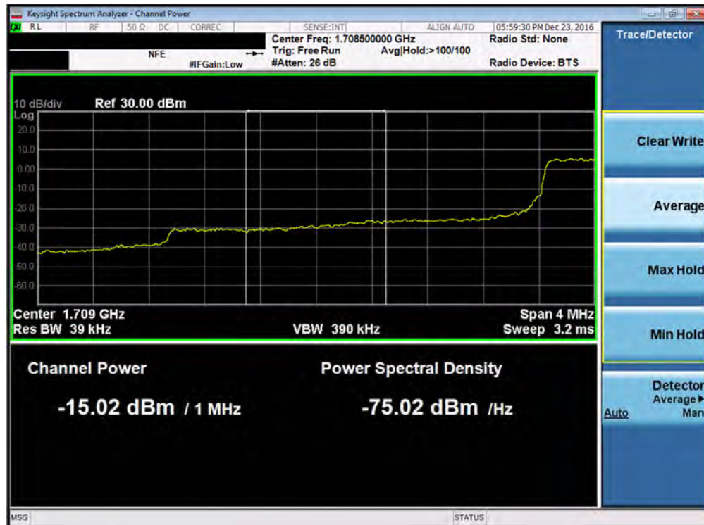
Plot 7-110. Lower Extended Band Edge Plot (Band 4 – 3.0MHz QPSK – RB Size 15)
