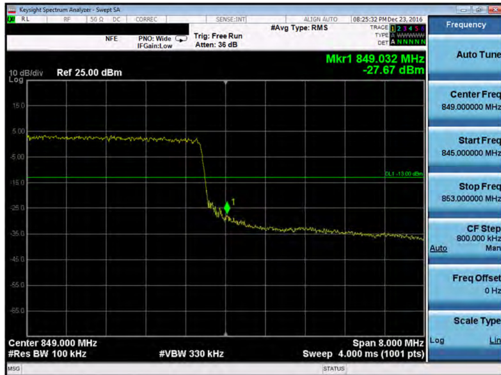
Plot 7-104. Upper Band Edge Plot (Band 5 – 10.0MHz QPSK – RB Size 50)
