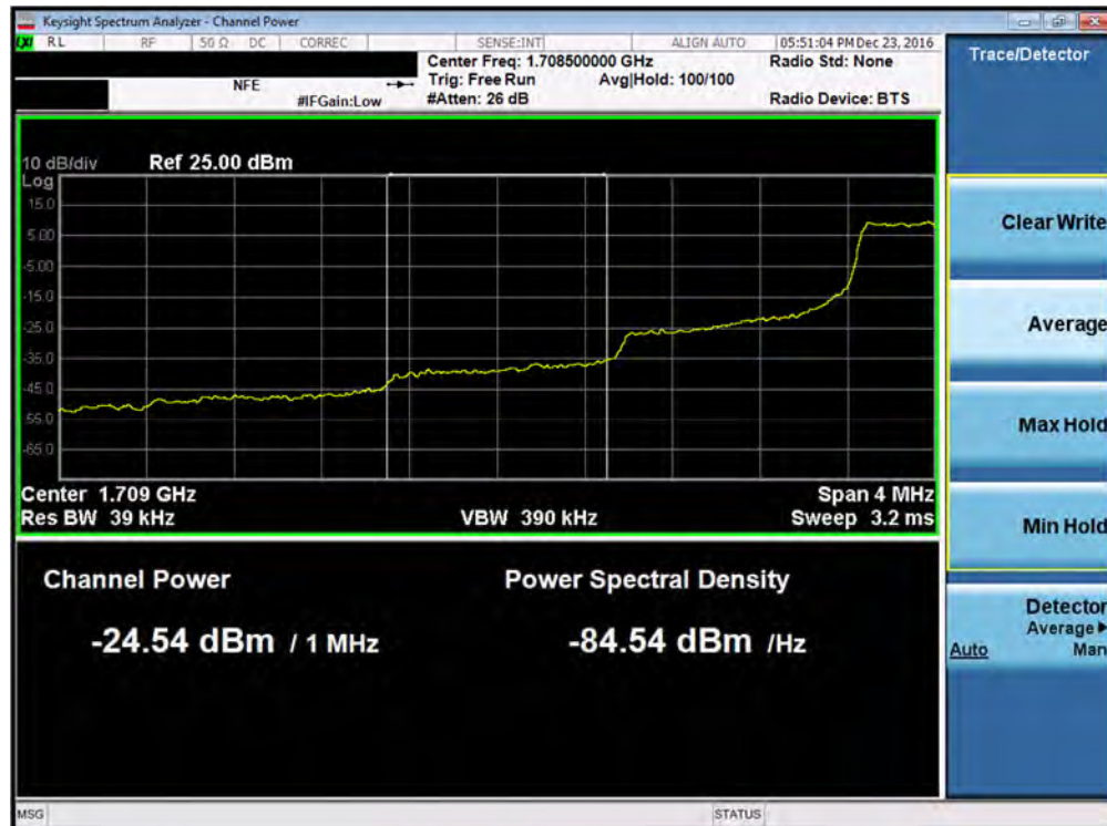
Plot 7-106. Lower Extended Band Edge Plot (Band 4 – 1.4MHz QPSK – RB Size 6)
