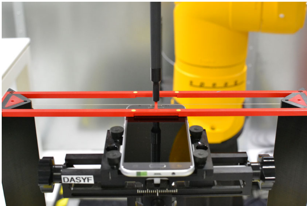
Figure 17-1 Ear Reference Point HAC Phantom Alignment
