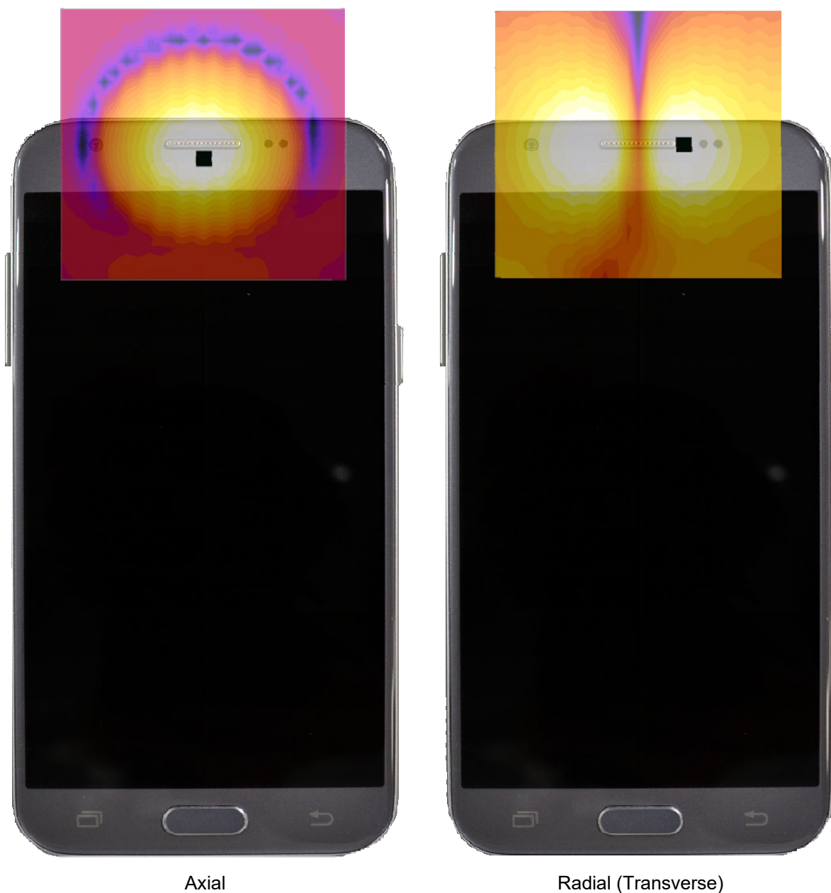
Figure 14-3 T-Coil Scan Overlay Magnetic Field Distributions
