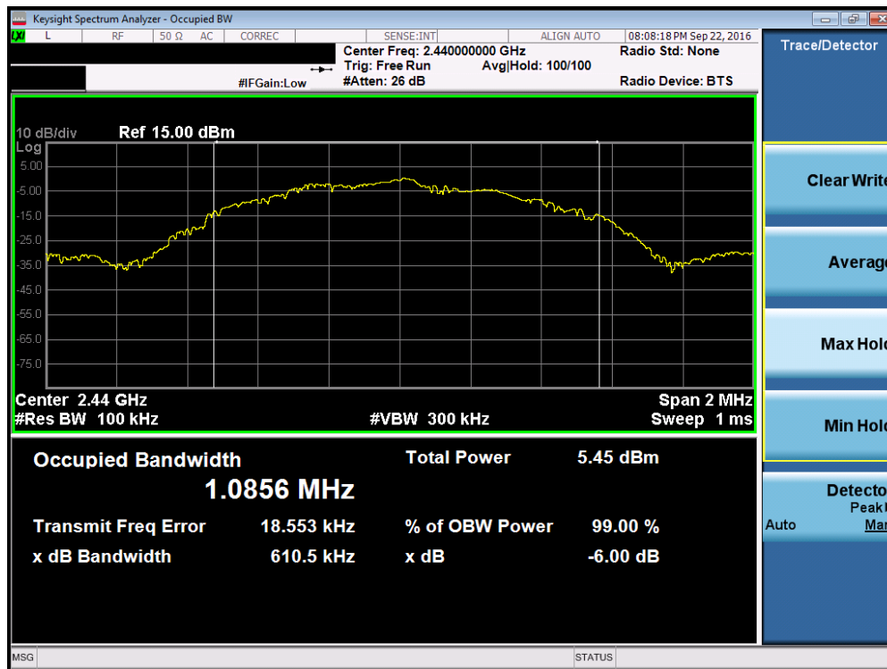
Plot 7-2. 6dB Bandwidth Plot (Bluetooth (LE) – Ch. 19)
