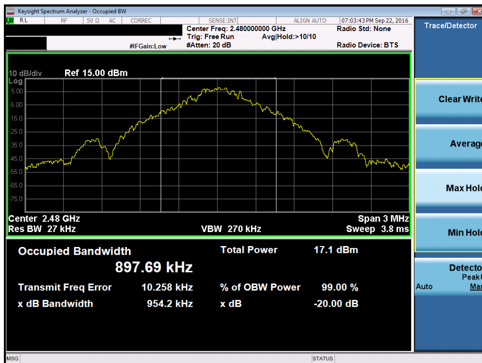
Plot 7-3. 20dB Bandwidth Plot (Bluetooth, 1Mbps – Ch. 78)
