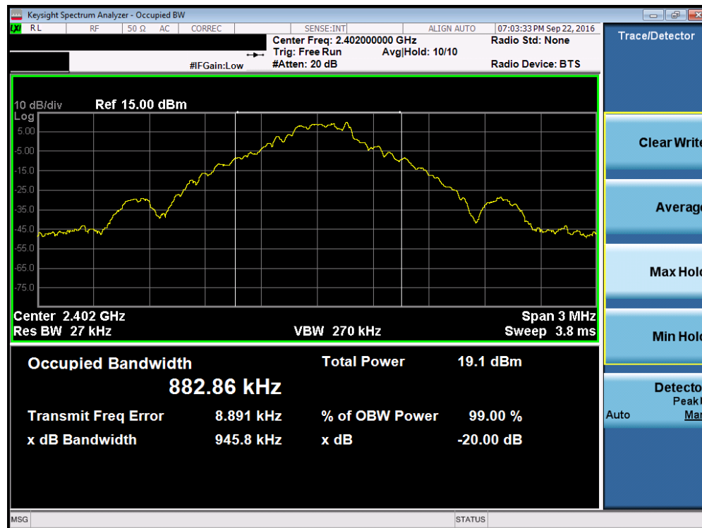
Plot 7-1. 20dB Bandwidth Plot (Bluetooth, 1Mbps – Ch. 0)
