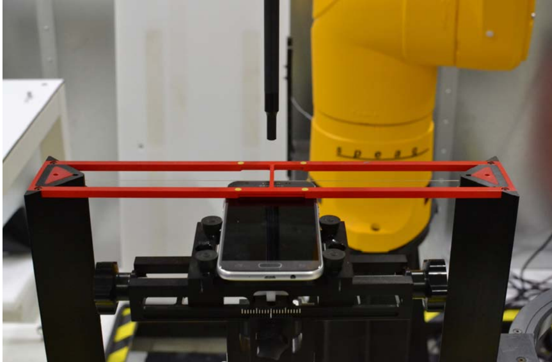
Figure 17-1 Ear Reference Point HAC Phantom Alignment
