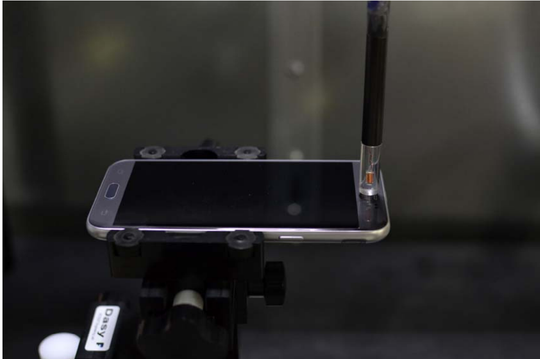
Figure 13-1 Test Setup for Wireless Device
