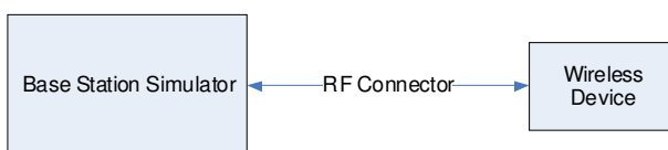
Figure 9-2 Power Measurement Setup
