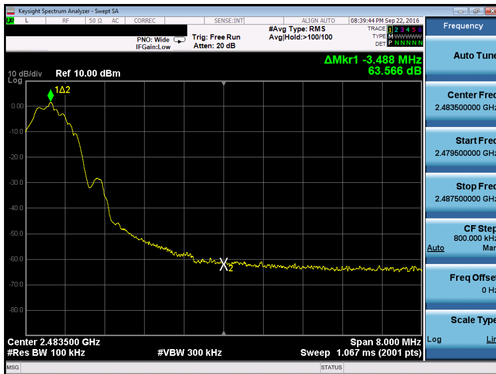
Plot 7-11. Band Edge Plot (Bluetooth (LE) – Ch. 39)
