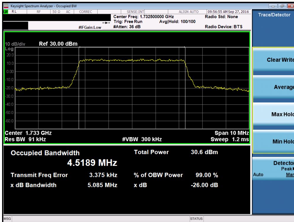
Plot 7-22. Occupied Bandwidth Plot (Band 4 – 5.0MHz 16-QAM – RB Size 25)
