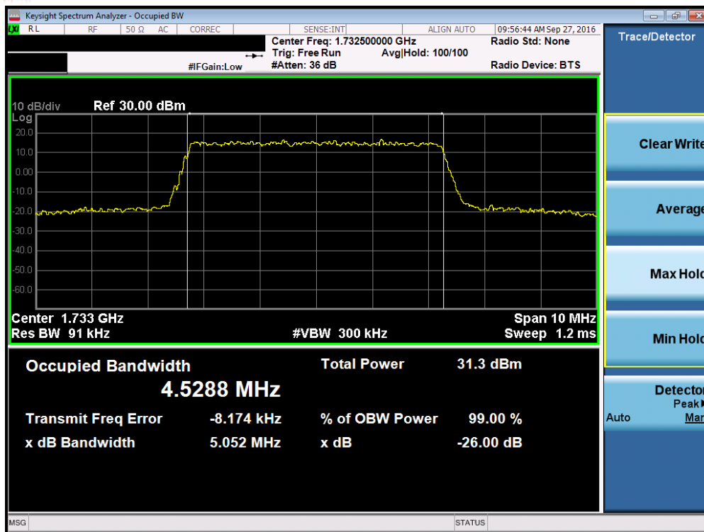
Plot 7-21. Occupied Bandwidth Plot (Band 4 – 5.0MHz QPSK – RB Size 25)
