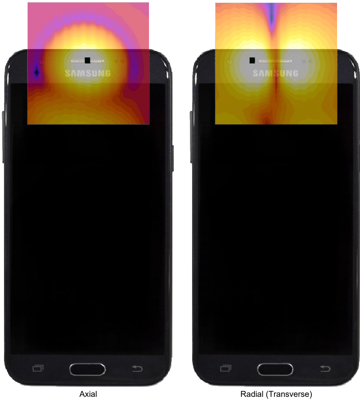
Figure 14-3 T-Coil Scan Overlay Magnetic Field Distributions
