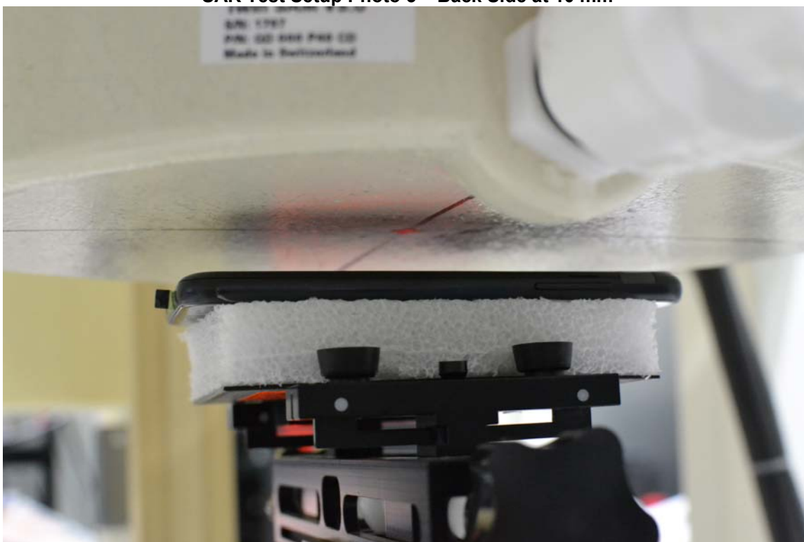
SAR Test Setup Photo 6 – Back Side at 15 mm
