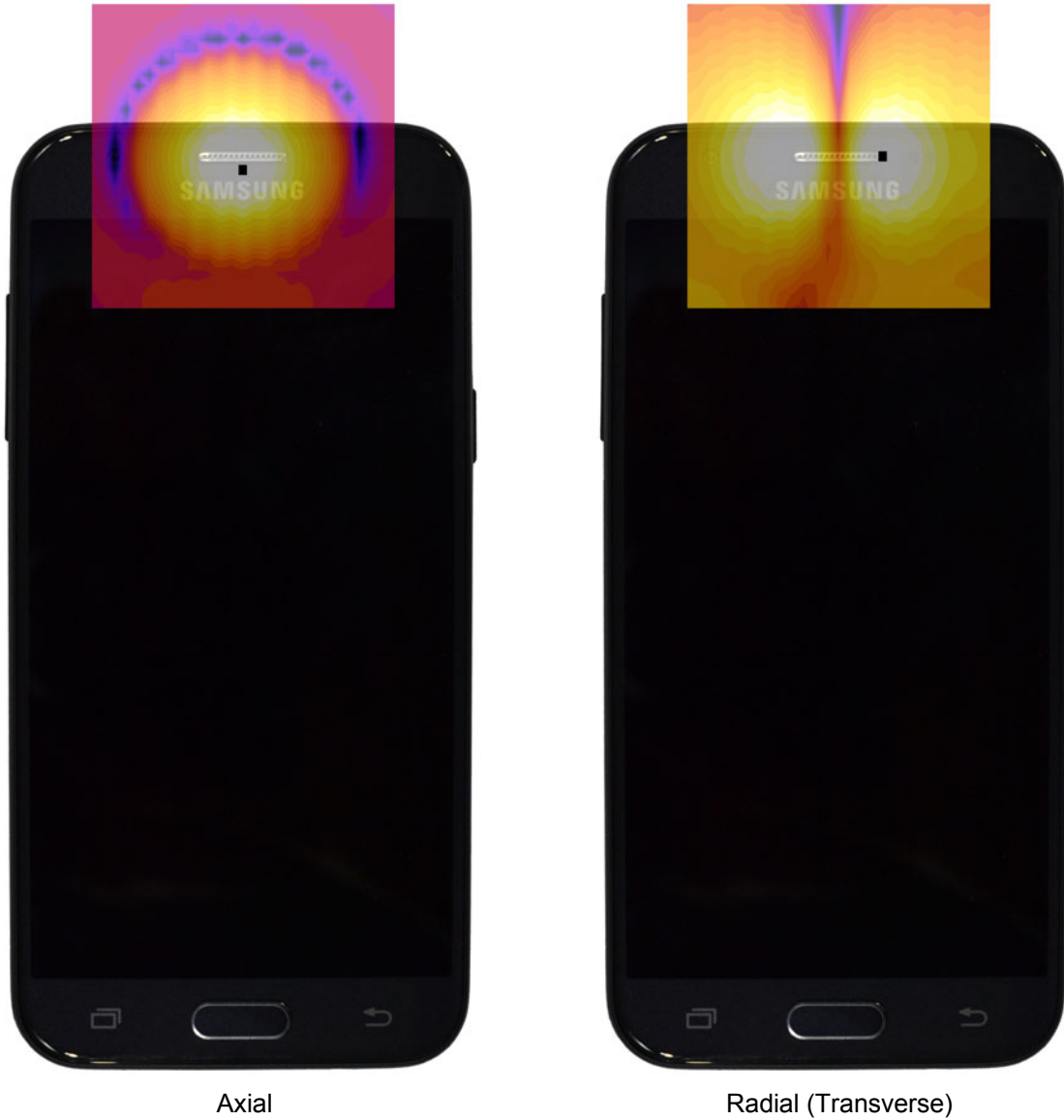
Figure 14-3 T-Coil Scan Overlay Magnetic Field Distributions
