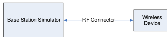
Figure 9-3 Power Measurement Setup
