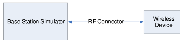
Figure 9-2 Power Measurement Setup
