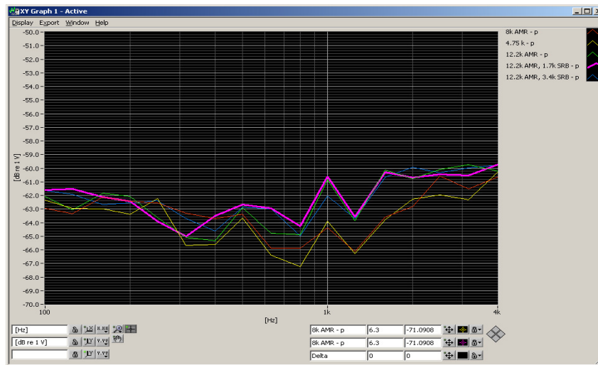
Figure 6-3 UMTS Audio Band Magnetic Noise
