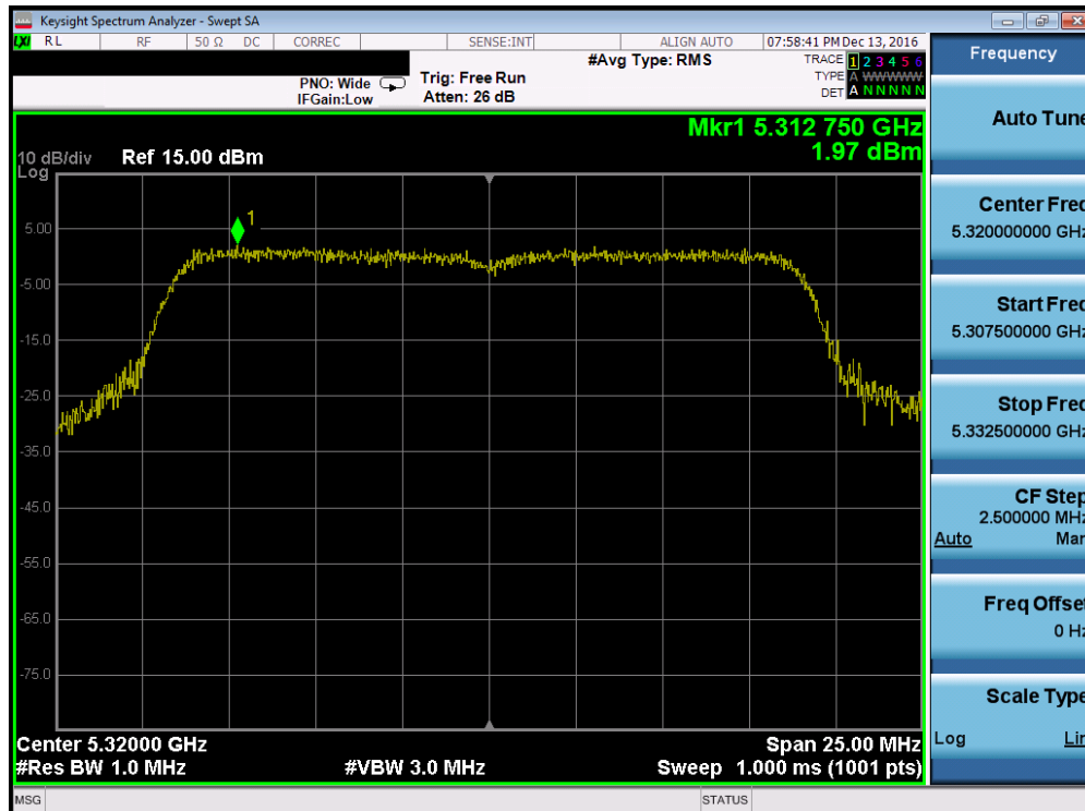
Plot 7-47. Power Spectral Density Plot (20MHz BW 802.11n (UNII Band 2A) – Ch. 64)
