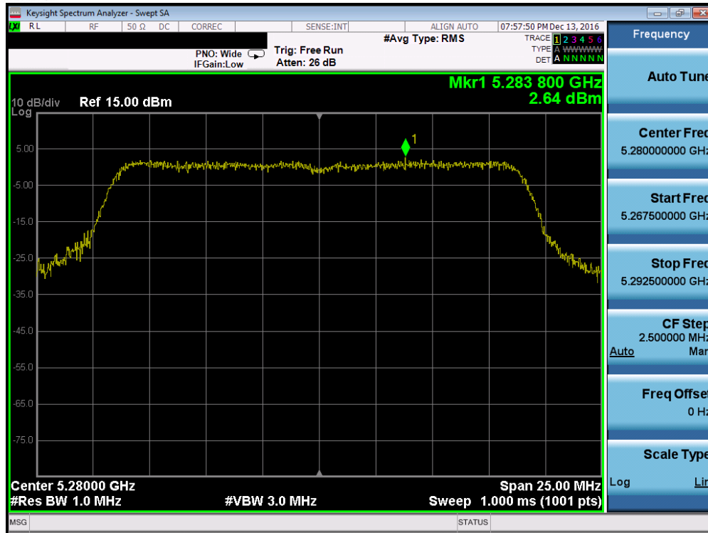
Plot 7-46. Power Spectral Density Plot (20MHz BW 802.11n (UNII Band 2A) – Ch. 56)
