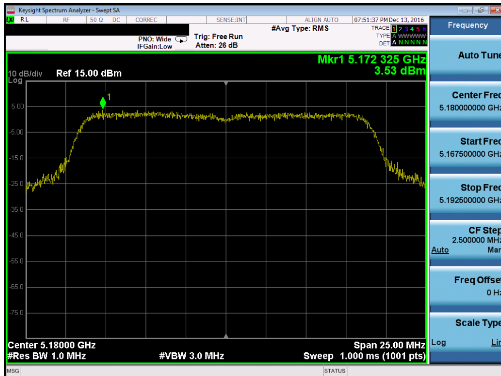
Plot 7-37. Power Spectral Density Plot (20MHz BW 802.11n (UNII Band 1) – Ch. 36)
