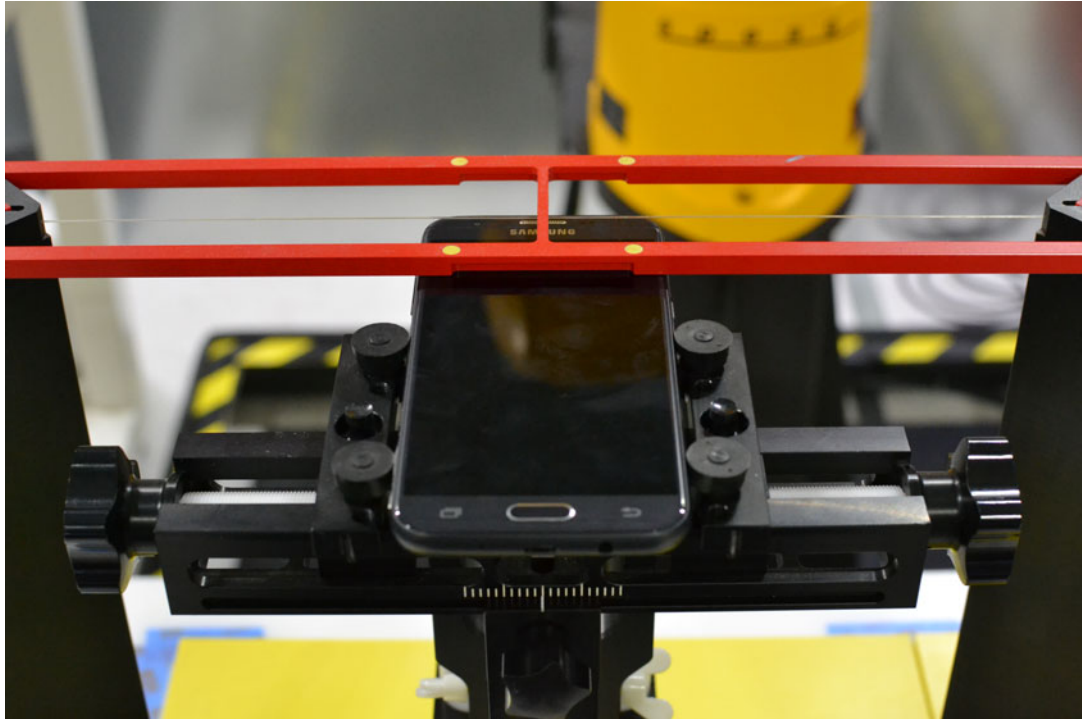
Figure 17-1 Ear Reference Point HAC Phantom Alignment
