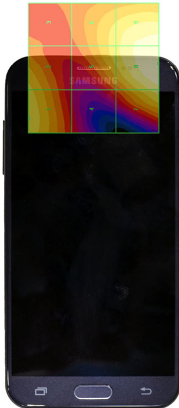
Figure 17-4 E-Field WD Scan overlay
