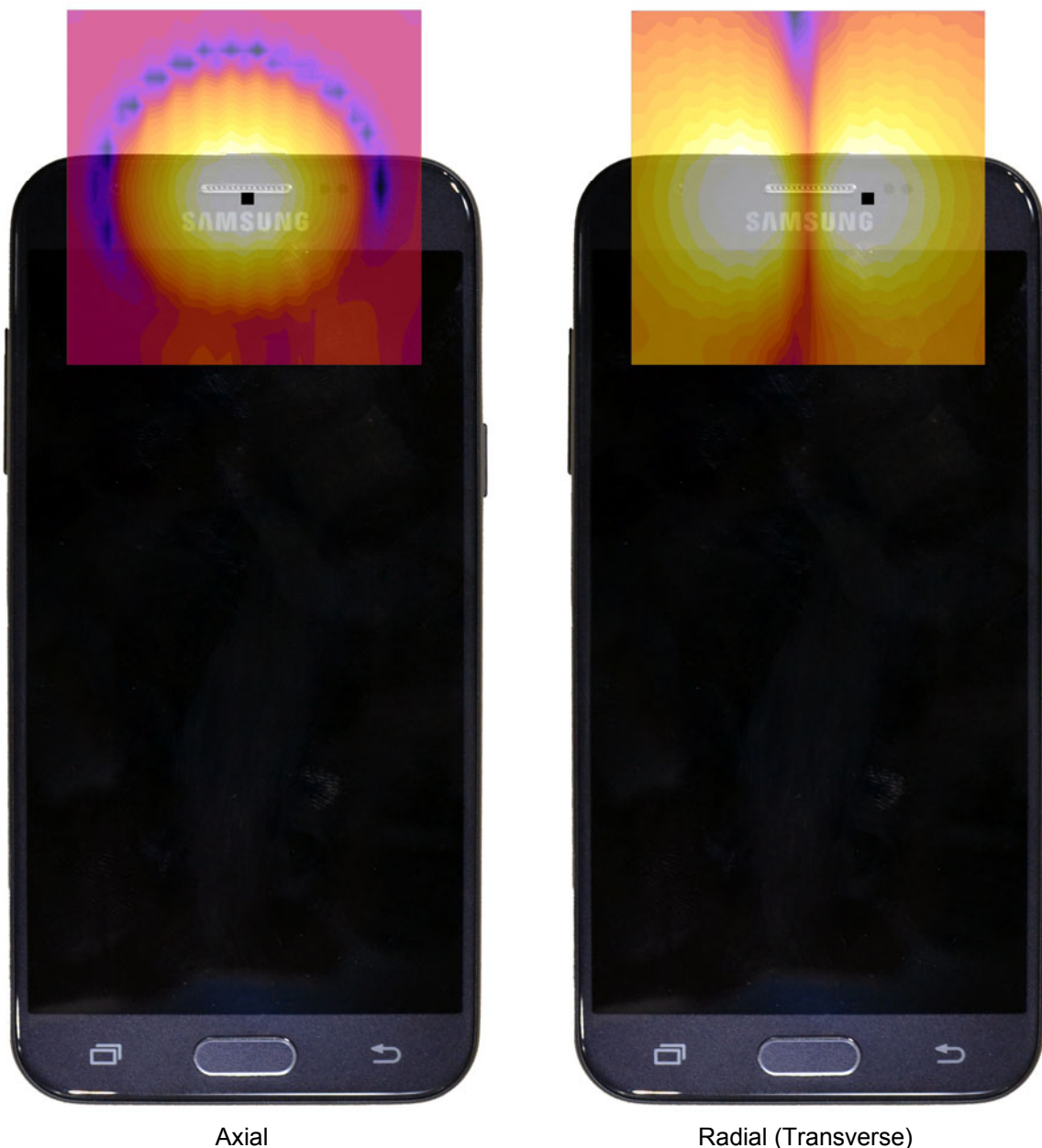
Figure 14-3 T-Coil Scan Overlay Magnetic Field Distributions
