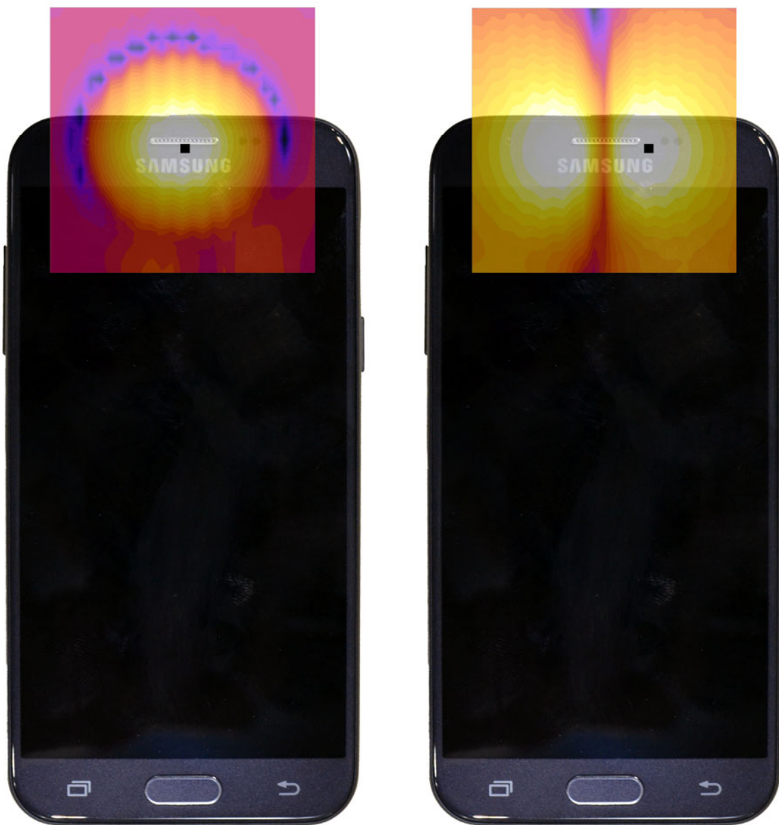
Figure 14-3 T-Coil Scan Overlay Magnetic Field Distributions
