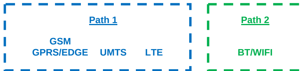
Figure 1-1 Simultaneous Transmission Paths
