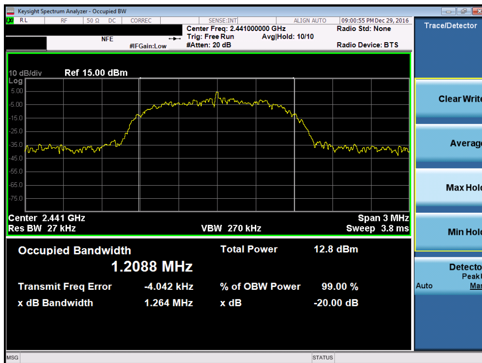
Plot 7-8. 20dB Bandwidth Plot (Bluetooth, 3Mbps – Ch. 39)
