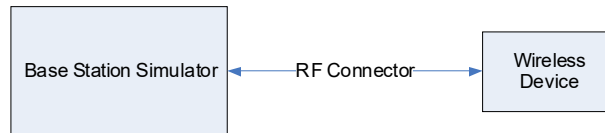
Figure 9-2 Power Measurement Setup
