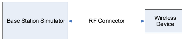
Figure 9-1 Power Measurement Setup
