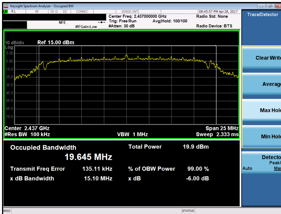
Plot 7-8. 6dB Bandwidth Plot (802.11n (2.4GHz) – Ch. 6)
