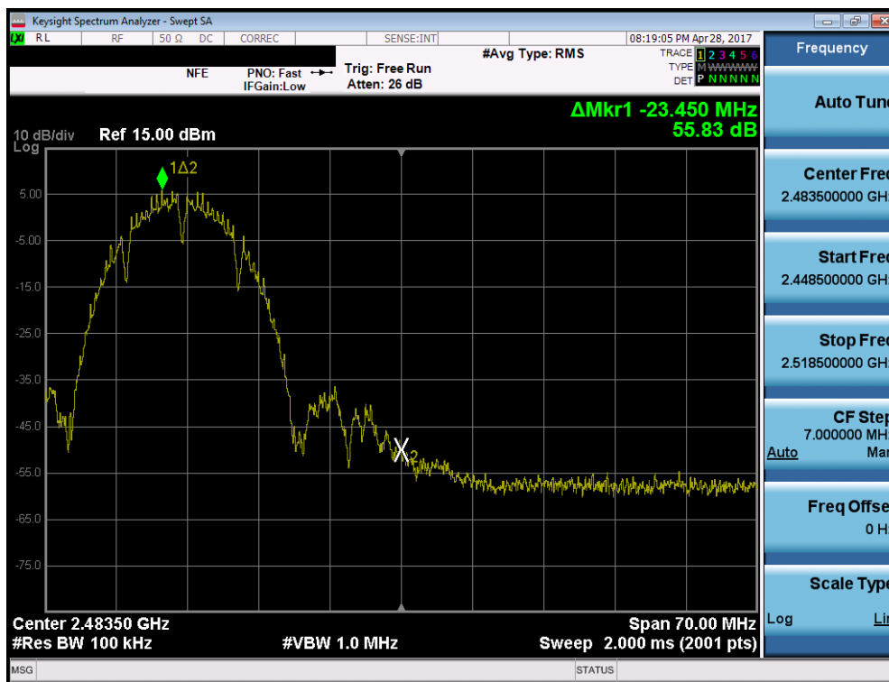
Plot 7-20. Band Edge Plot (802.11b – Ch. 11)
