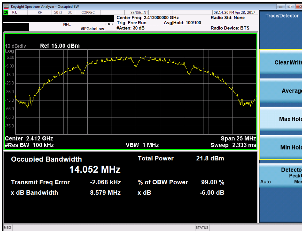
Plot 7-1. 6dB Bandwidth Plot (802.11b – Ch. 1)
