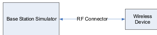
Figure 9-3 Power Measurement Setup
