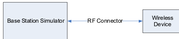
Figure 9-3 Power Measurement Setup
