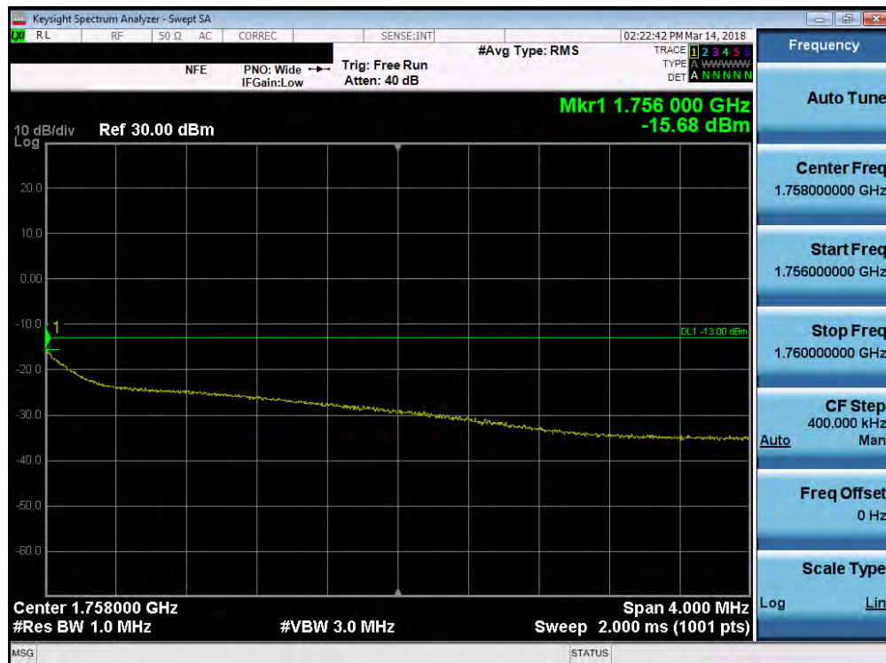
Plot 7-92. 4MHz Span Plot (AWS WCDMA Mode - High Channel)
