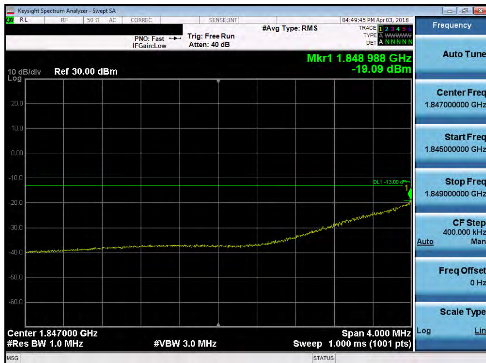
Plot 7-84. 4MHz Span Plot (PCS CDMA Mode - Low Channel)
