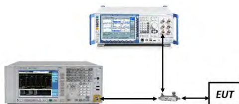
Figure 7-1. Test Instrument & Measurement Setup
