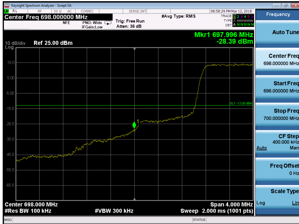
Plot 7-113. Lower Band Edge Plot (Band 12 - 1.4MHz QPSK - Full RB Configuration)
