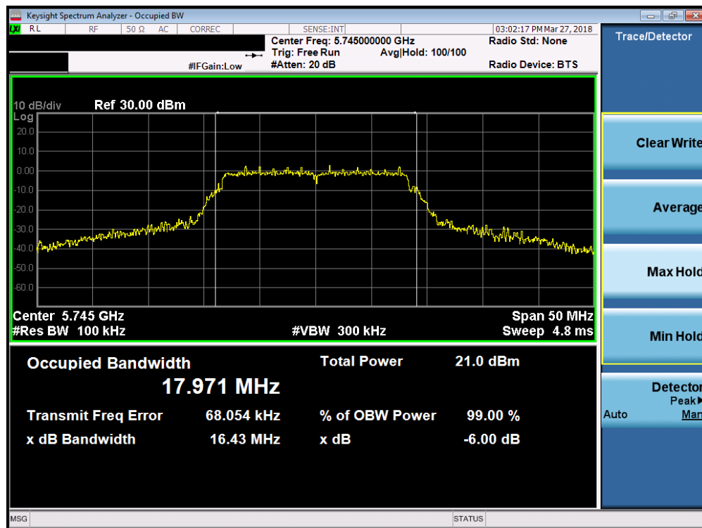
Plot 7-26. 6dB Bandwidth Plot (802.11a (UNII Band 3) – Ch. 149)
