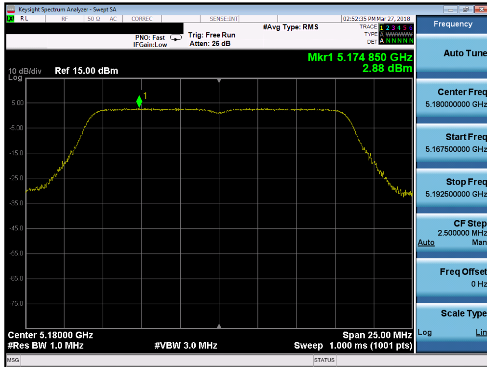
Plot 7-34. Power Spectral Density Plot (802.11a (UNII Band 1) – Ch. 36)
