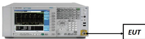
Figure 7-4. Test Instrument & Measurement Setup
