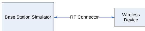
Figure 9-1 Power Measurement Setup
