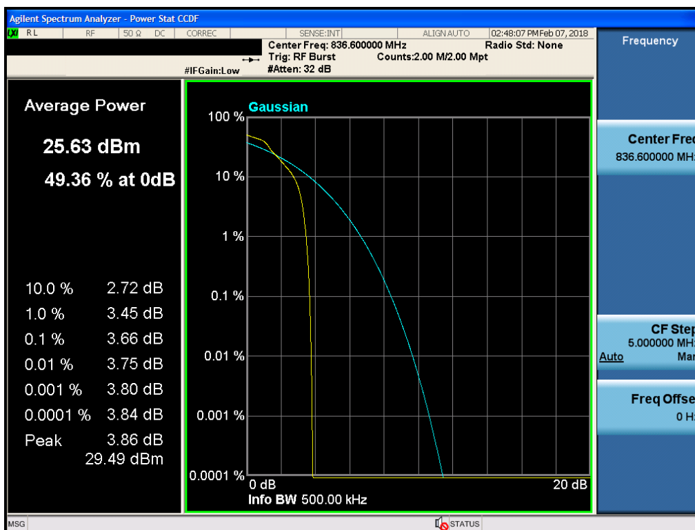
Plot 7-70. Peak-Average Ratio Plot (EDGE850 Mode)
