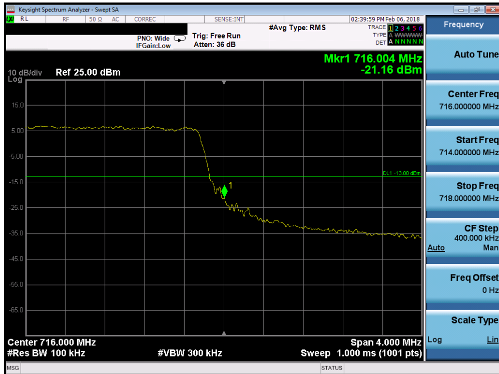
Plot 7-125. Upper Band Edge Plot (Band 12 - 5.0MHz QPSK - Full RB Configuration)
