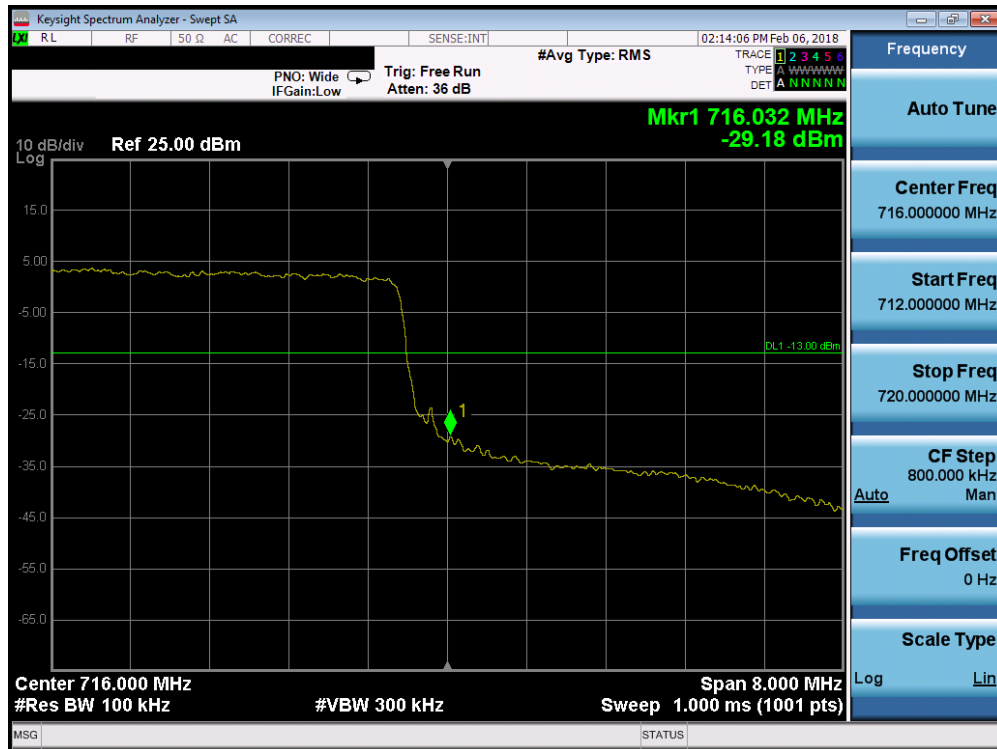
Plot 7-127. Upper Band Edge Plot (Band 12 - 10.0MHz QPSK - Full RB Configuration)
