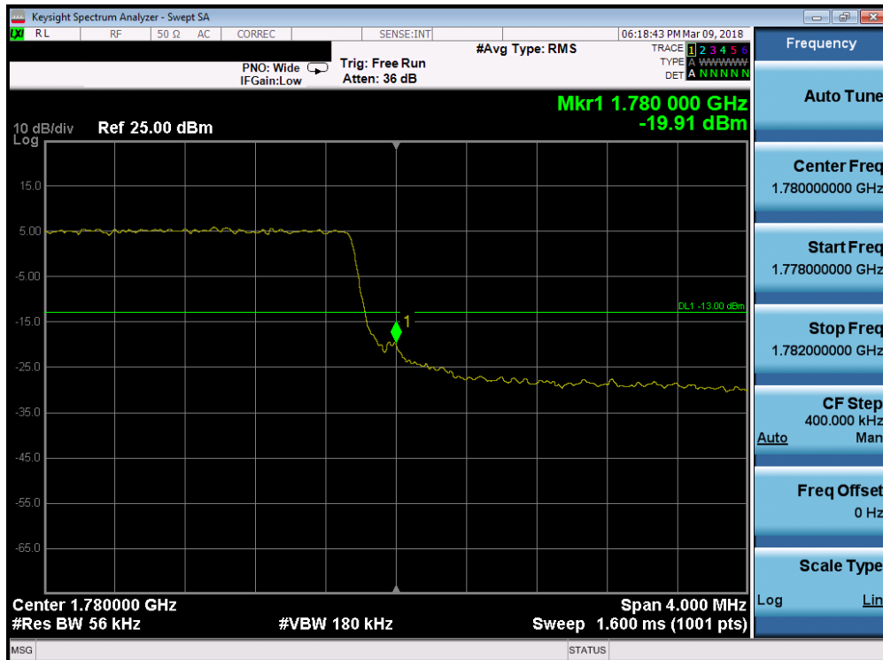
Plot 7-148. Upper Band Edge Plot (Band 66 - 5.0MHz QPSK - Full RB Configuration)
