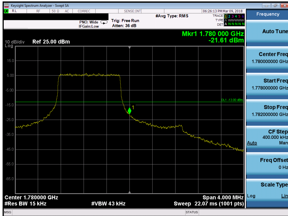
Plot 7-140. Upper Band Edge Plot (Band 66 - 1.4MHz QPSK - Full RB Configuration)
