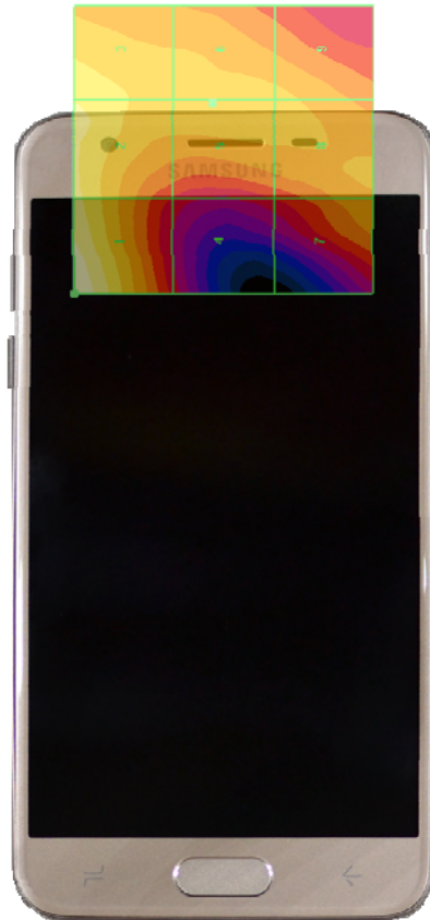
Figure 17-4 E-Field WD Scan overlay
