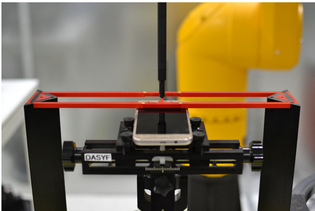
Figure 17-1 Ear Reference Point HAC Phantom Alignment
