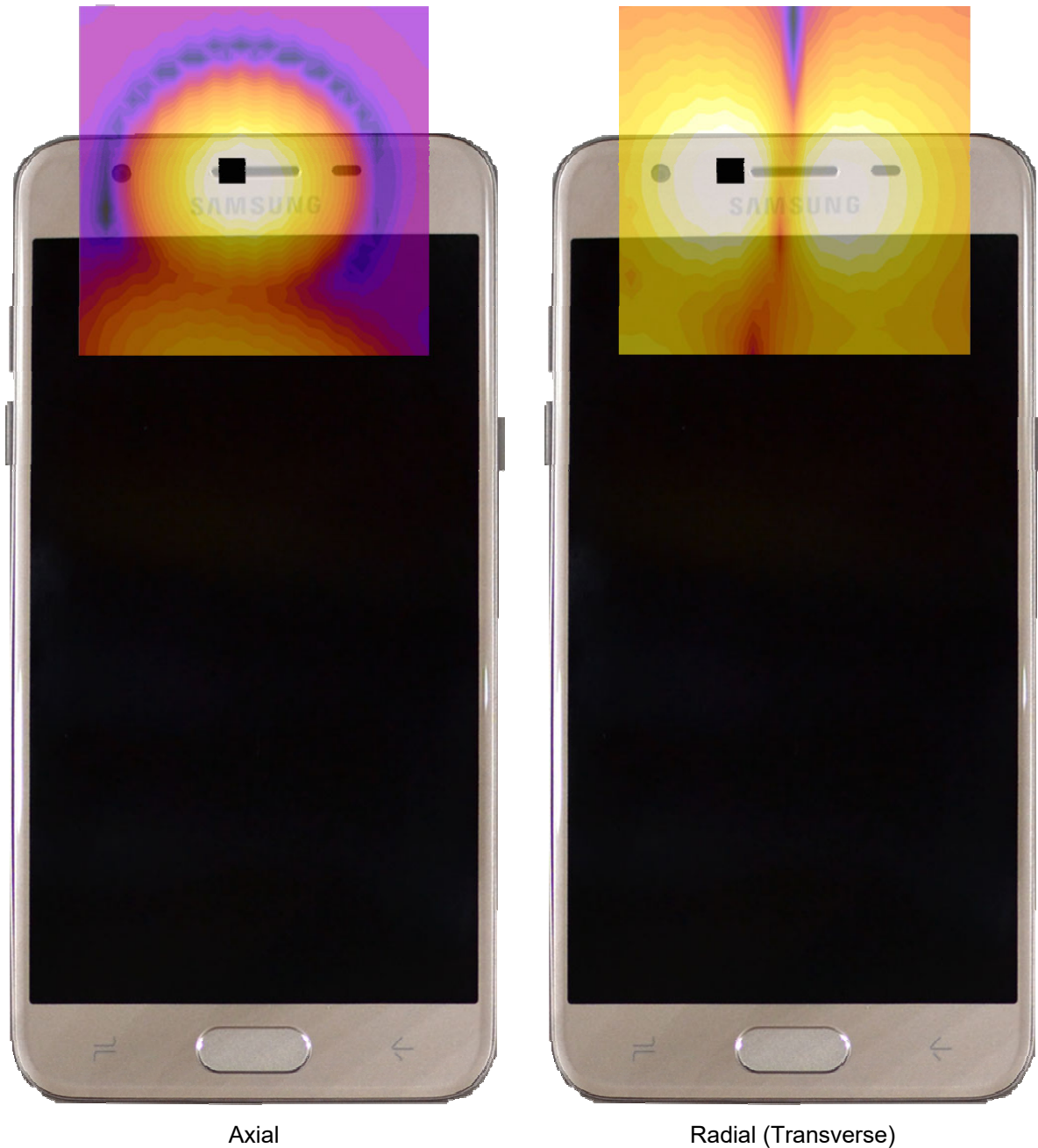
Figure 16-3 T-Coil Scan Overlay Magnetic Field Distributions
