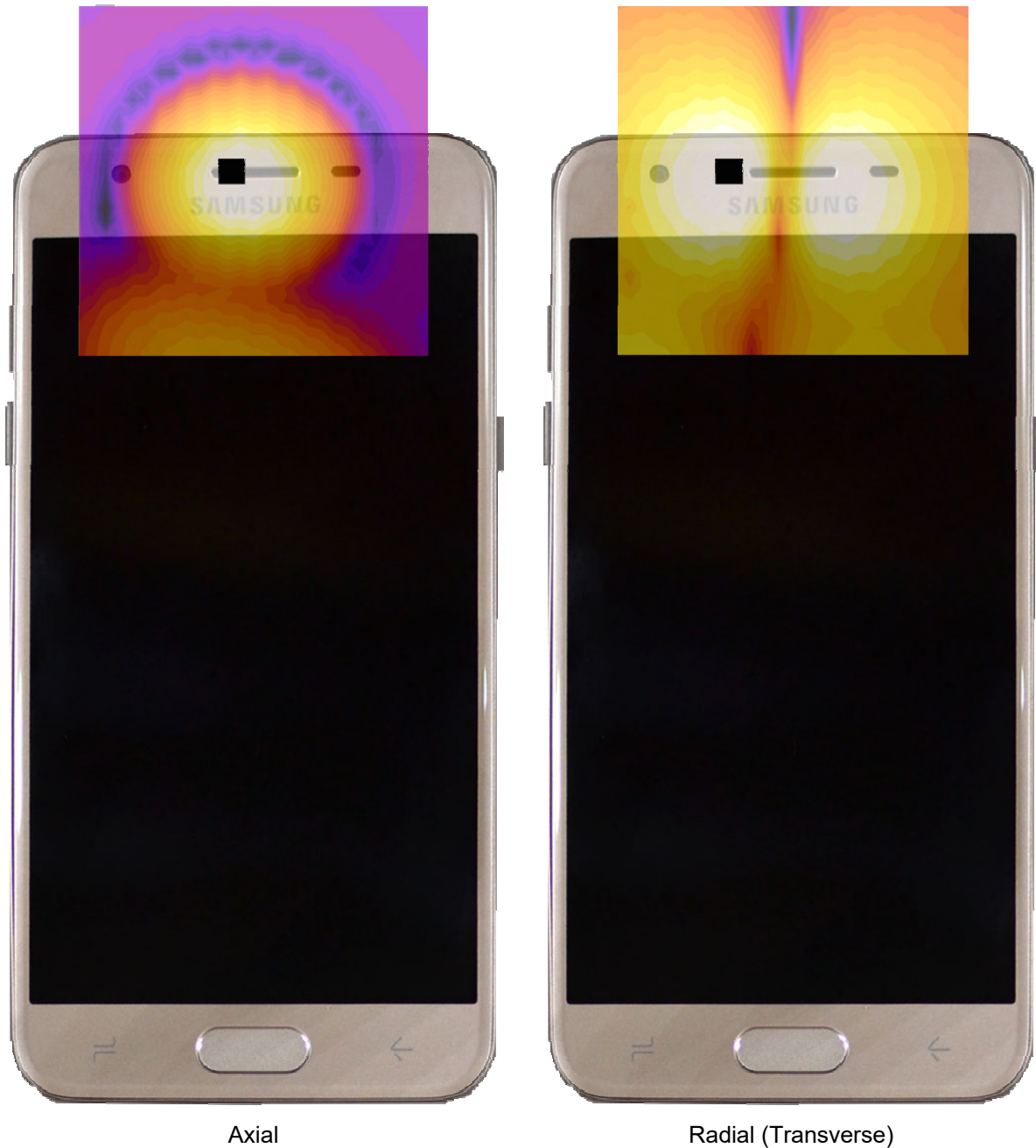
Figure 12-3 T-Coil Scan Overlay Magnetic Field Distributions
